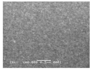
**Figure3.** SEM surface morphology of Ni /Si (sample2)
