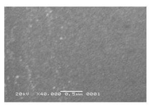
**Figure 4.** SEM surface morphology of Ni/Si (sample3)
