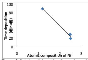
**Figure 5.** Relation of deposition time and Atomic composition of Ni
