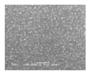
**Figure2.** SEM surface morphology of Ni /Si (sample1)
